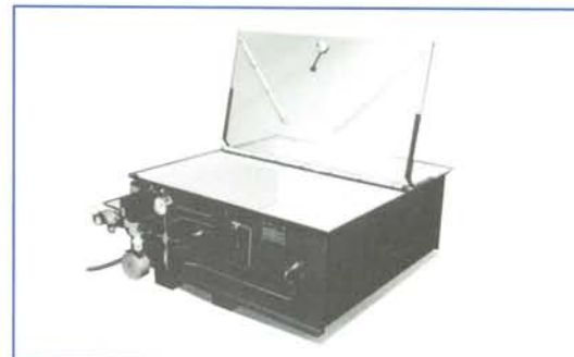
A test rig with a test chamber up to 48" square for testing hose coils for pressures up to 30,000 psi
