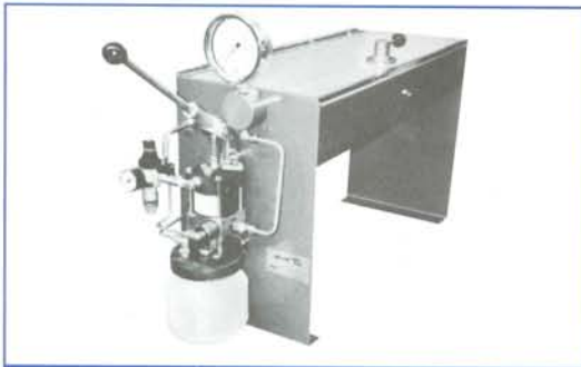
A small portable, single station, low cost, manual or air operator test rig for small hose lengths and pressures up to 15,000psi
