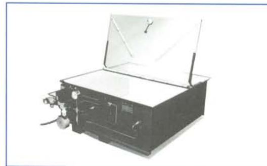
A test rig with a test chamber up to 48" square for testing hose coils for pressures up to 30,000 psi
