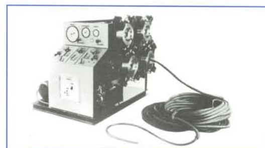
Mandrel extraction and pressure test rig combines high flow with testing to 30,000 psi
